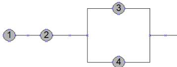
Consider a system consisting of four components, and suppose that the system functions if and only if components 1 and 2 both function and at least one of components 3 and 4 function. Its structure function is given by
